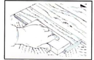
Secure your starter rows with a straight edge (2x4's). Once the remainder of the floor has been installed go back to the beginning and remove the straight edges and spread adhesive on the remainder of the open subfloor. Remember planks closest to the wall may have to be scribed and cut to fit due to irregularities along the wall. When using Mohawk's Pro-Tack M908 adhesive it is not necessary to roll the floor.
